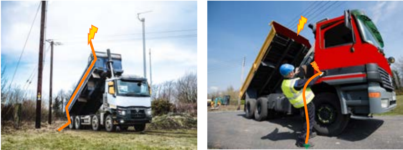
Figure 1: The path of electrical current flowing to earth for a truck in contact or near contact with overhead lines
