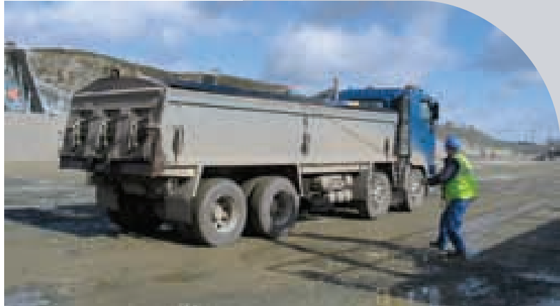
Sheeting from ground level
