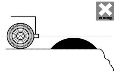
Edge protection less than either 1.5 metres, or the radius of the vehicle wheel, or with sloping sides makes an ideal ramp for the vehicle to run over, and is totally ineffective.
