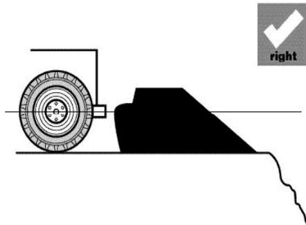
Rocks can be used if they can safely absorb the impact, for example by heaping materials like scalplings between and behind the rocks to provide an adequate barrier. A violent stop due to impact with large rocks would, of course, increase the risk of injury to the driver, and of damage to the vehicle, and so should be avoided.
