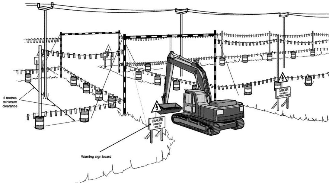
If work needs to be carried out below power lines and it is possible that cranes, excavators or other vehicles, could reach into the danger zone, the lines should normally be isolated and earthed before work begins. If this is not feasible, physical safeguards such as chains on the booms may be required to prevent vehicles reaching into the danger area. If in doubt, advice should be obtained from the electricity company.
