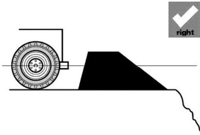
A bank of unconsolidated material like scalplings is suitable if it is big enough to allow the vehicle's momentum to be absorbed. The impact face needs to be as nearly vertical as possible and the height as described above.
