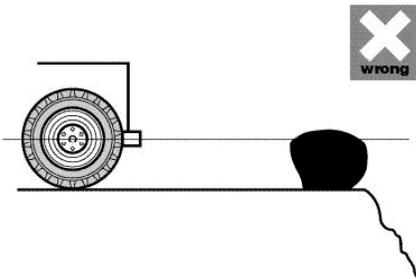
Blocks of stone placed along the edge of a bench, ramp or roadway, which can be easily pushed out of the way by a vehicle, are not suitable for edge protection.
