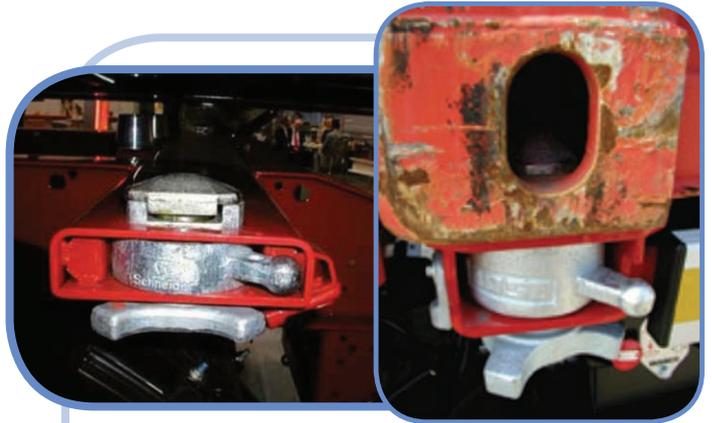
Figure 4. Twist locks fitted and in operation
