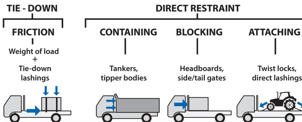
Figure 2. Load restraint methods (To control forward + rearward motion)
