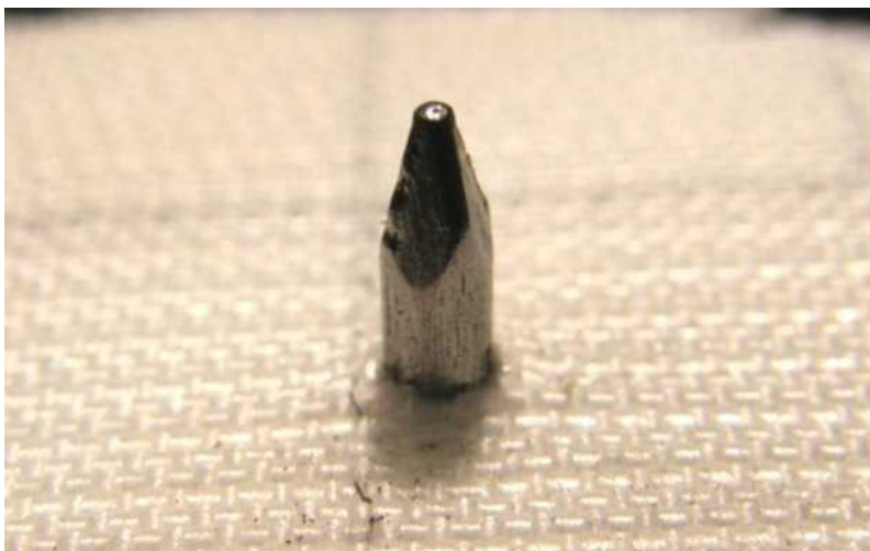
Image 1: Nail in non-metal insert
