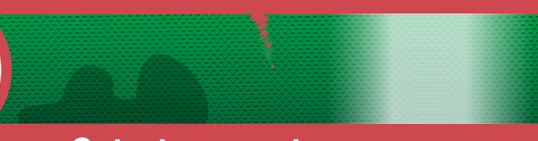
Cuts, tears, water, rock salt and oil contamination can lead to straps wearing out.
