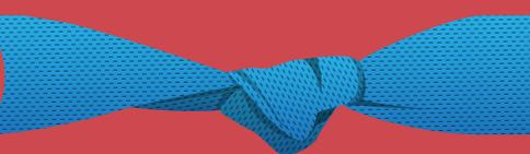
Never use a knot in any part of the strap that's under tension.
