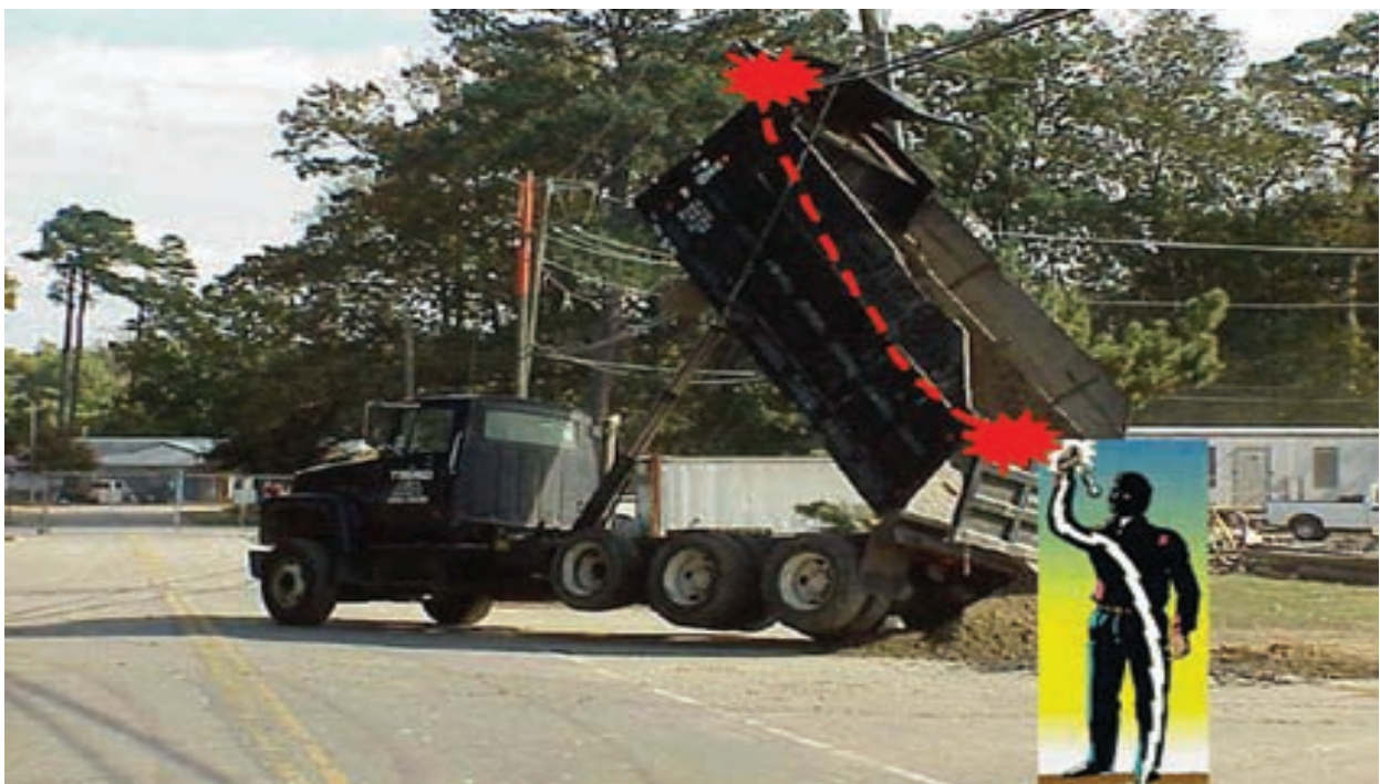
Fig 1 Path of electric current flowing to earth for a truck in contact or near contact with overhead line.
