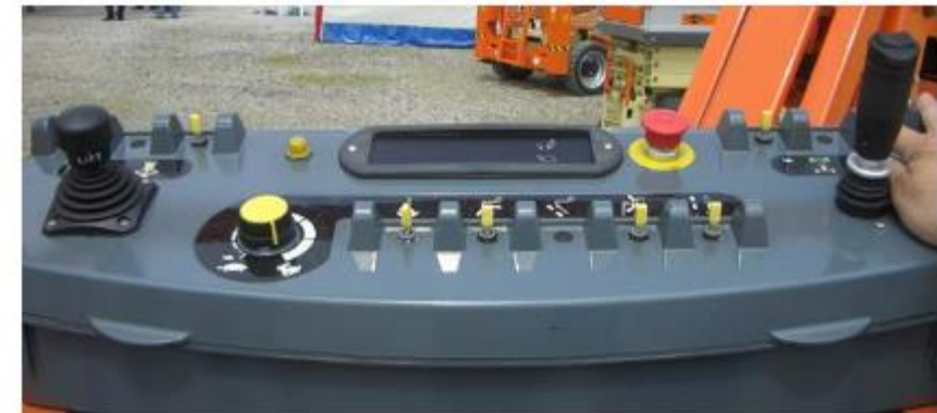
Photograph 2 - Platform control panel for another articulating boom
