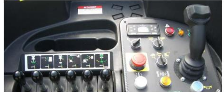
Photograph 1 - Platform control panel for an articulating boom
