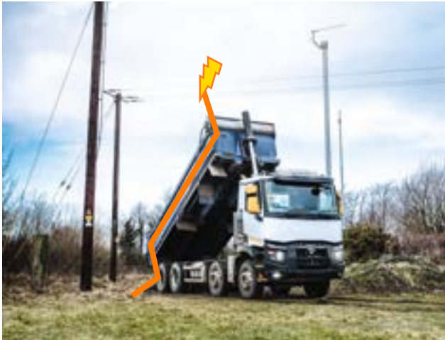
Figure 1: The path of electrical current flowing to earth for a truck in contact or near contact with overhead lines
