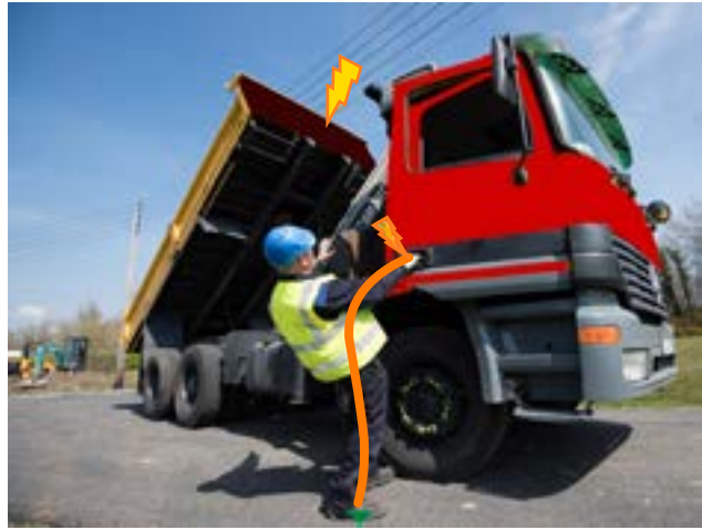
Figure 1: The path of electrical current flowing to earth for a truck in contact or near contact with overhead lines
