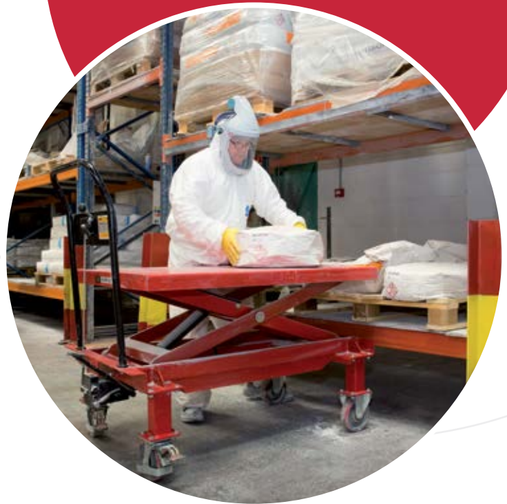
After: Operative slides bag onto a scissors lift table
