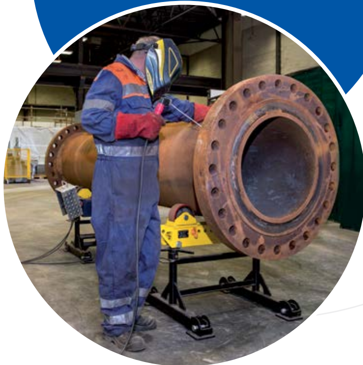
After: Rollers in position to allow operator maintain good posture while welding pipe
