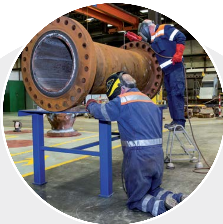
Before: Operators carrying out welding work while maintaining awkward positions
