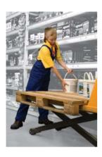
Using truck with height regulation for placing goods on racks.
