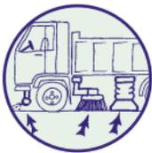
Excessive amounts of dust can cause eye and respiratory irritation. In general dust and muck is a nuisance for both workers and others in the vicinity. All traffic routes in public areas adjacent to demolition works should be kept clear of muck. During dry periods the routes should be dampened to keep dust down.
