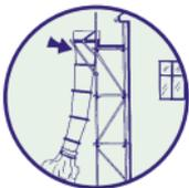
Chutes should be used for discarding materials, materials should never be thrown from scaffolding or windows etc. The Chute should extend down into a waste skip. Exclusion zones under the drop zones should always be created where construction materials and debris is discarded.
