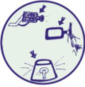
With plant that has restricted visibility, particularly while carrying out reversing operations suitable warning devices, or sight seeing devices must be fitted e.g. CCTV, flashing beacons, convex mirrors etc.
