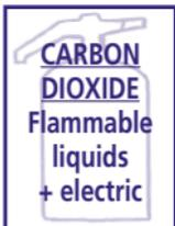
Carbon dioxide extinguishers can be used on fires involving flammable liquids or electrical apparatus. Carbon dioxide should not be used in confined spaces where there is a danger that the fumes can be inhaled.
