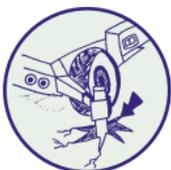
The ground area on which any demolition plant is to be used should be examined to ensure that it is capable of taking the applied loads. Expert advice may be necessary.
