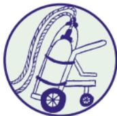
Gas bottles on site, must always be stored upright, and chained to prevent inadvertent falling.
