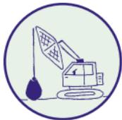
This method breaks down the building or structure by swinging a weight, usually in the shape of a ball, from a crawler crane, which should be fitted with a lattice jib. This weight is then released to impact the structure, repeatedly, in the same or different locations. Care must be taken so that the ball is not trapped, as a trapped ball can cause
