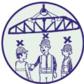
Work should never take place directly above other workers. Where overhead work is likely to occur, adequately sized exclusion zones should be created to ensure that persons are not at risk from falling objects.
