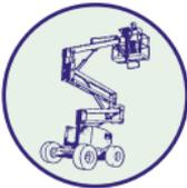
A Boom Hoist has an extendable folding boom with cage attached, it can be used for work at height if the ground conditions are suitable. Boom hoists can also be used to gain access to remote areas. Selection must be based on suitability for the task, the manufacturers guidelines for safe use must be followed fully. Only competent and trained operators should control the movement of these hoists. Other vehicles should be strictly controlled in the vicinity of hoists.
