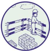
All materials should be stored where they cannot fall on to workers below. Materials should be kept tidy and stable making sure that all access routes are kept clear. Working platforms should not be cluttered or blocked with materials, there must always be adequate space for safe access. All loose materials should be removed on an ongoing basis.
