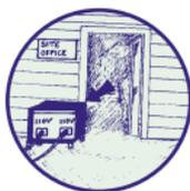
To avoid the silent killer, petrol and diesel driven generators must always be used outdoors to avoid the deadly effects of carbon monoxide build up from exhaust gases.
