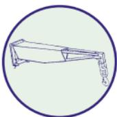
Chains and slings must not be wrapped around the forks of a teleporter when lifting a load. When required to lift loads with a teleporter, the forks should be removed and a crane extension with hook or shackle should be used.
