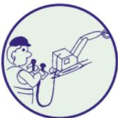
Is the operation of machines remotely, e.g. using “umbilical” cable control or robotic devices. Any machine used must be maintained in good working condition and be appropriate for the task having regard to the environment and its location. Where machines are used the supporting surfaces must be strong enough to support such machines and any associated loads.
