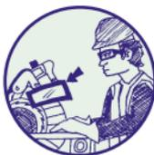
Many hand/portable tools have rotating shafts and components, others due to their application will emit fragments including dust and sparks. Such tool must have suitable guards fitted, e.g. circular saw guards, power-take-off shaft guards etc.
