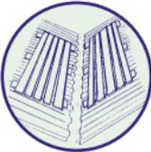
If required to work on or access on fragile roofs including work adjacent to roof lights, crawling boards may be used, they are intended to spread load such that point load does not exceed the load which may result in such roofs breaking. The selection of suitable crawling boards for particular use should be made by competent persons.
