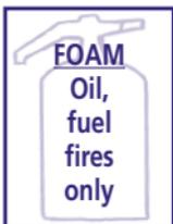
Foam extinguishers are suitable for most fires involving flammable liquids. Where the liquid on fire is in a container, direct the jet at the inside edge of the container or at an adjoining vertical surface above the level of the burning liquid. This breaks the jet and allows the foam to build up and flow across the surface of the liquid to smother the fire. Do not aim the jet directly into the burning liquid.
