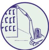
High and ultra high reach machines fitted with suitable booms and arms used with concrete pulverizers and combination attachments should be considered for the demolition of high rise buildings. When using such machines the correct position relative to the work face must be maintained and that the angle of the boom is in accordance with the manufacturer's recommendations to ensure safe operation and stability of the machine.
