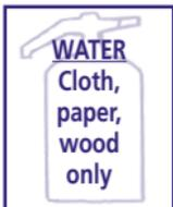
Water fire extinguishers are used for cloth, paper and wood only. Direct the jet at the base of the flame and keep it moving across the area of the fire.
