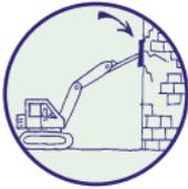
Involves the use of a machine fitted with a pusher arm exerting a horizon thrust. Used in progressive demolition, where the height of the structure is reduced by pushing over small sections. The point of contact of the arm with the wall must be at an appropriate distance below the top of the wall. Prior to use the assembled machine must be inspected by a competent person, to ensure that the attachment is secure and that all connections are fitted correctly and free from defects.
