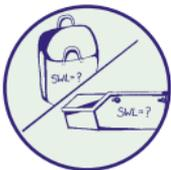
All skips and bins must be appropriate for the task and if used as lifting gear when attached to lifting appliances all lifting lugs and lifting eyes must have their safe working load (SWL) clearly visible. Always check the SWL before lifting commences. When used as lifting gear, such bins and skips must be certified as appropriate.
