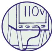
All portable electric tools rated below 2 kilowatts used on construction and demolition sites must be rated at 110V.
