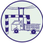
Burns and electrocution can result if raised tipper truck bodies, cranes or excavators touch or come close enough to overhead power lines to cause arcing. Never work close to, or access close to or under live overhead lines when lifting. Refer to ESB guidance booklet.
