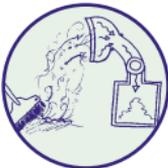
Local exhaust systems removes dust directly from the area in which it is produced
