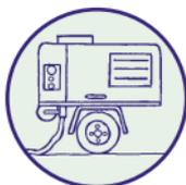
Compressors must be maintained and serviced on a regular basis. All connections and flexible hosing used must be in good condition and replaced if damaged. All guards must be secured before starting, such that there are no exposed rotating pulleys or belts.
