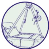
A tripod is a standard piece of rescue equipment for persons working in confined space, employee can be lowered into confined space by a "buddy", and more importantly can be raised out of the confined space, using a tripod.
