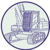
Cabs of demolition plant must be sufficiently protected to prevent falling materials crushing or penetrating into the occupied zone.
