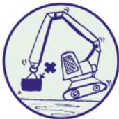
Lifting appliances and lifting gear should never be used to lift beyond their stated safe working load. This is the maximum load as assessed by a competent person which an item of lifting equipment may raise, lower or suspend under the particular service conditions.
