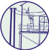
Contact with overhead lines can kill. Never erect scaffolding close to or under overhead lines. Never work close to, or access close to, or under overhead lines.
