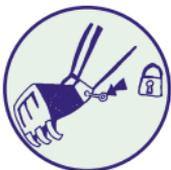
Ancillary equipment used in connection with demolition and lifting equipment must at all time be secured. This may require the insertion of locking pins, to prevent inadvertent dropping of the attachment.
