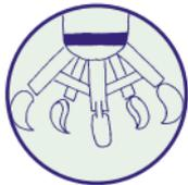
A grapple is designed for use in both demolition and handling applications. The jaws interlock to enable partial loads to be safely secured. Prior to use the assembled machine must be inspected by a competent person, to ensure that the attachment is secure and that all connections are fitted correctly and free from defects.
