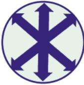
The bursting agent (e.g. expansion gas, expanding chemicals, hydraulic pistons or wedges) is inserted into a prepared cavity in the structure to be demolished. Upon being energised the increase in the resulting pressure causes fractures that propagates through crevices leading to structure rupture. Bursting techniques can be used for demolition of concrete or rock, especially where reduction of noise, dust and vibration need to be taken into account.
