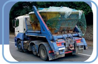
Skips must not be overloaded or exceed the safe load capacity of the skip lorry.
