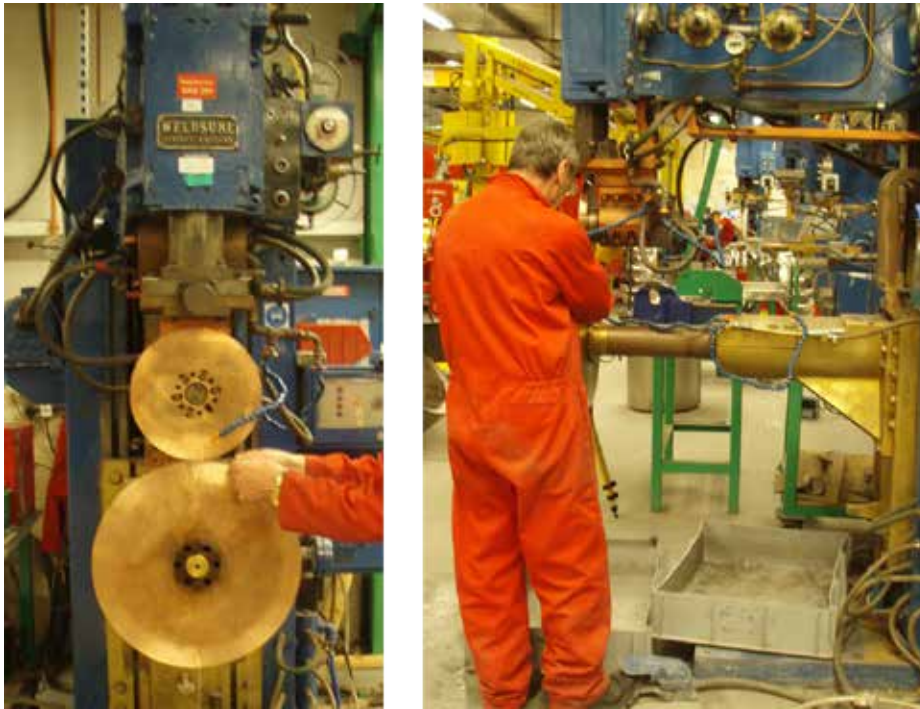
Figure 7.3 — Seam welder front and side views
