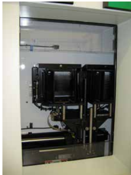
Figure 9.1 — Wafer loading area
