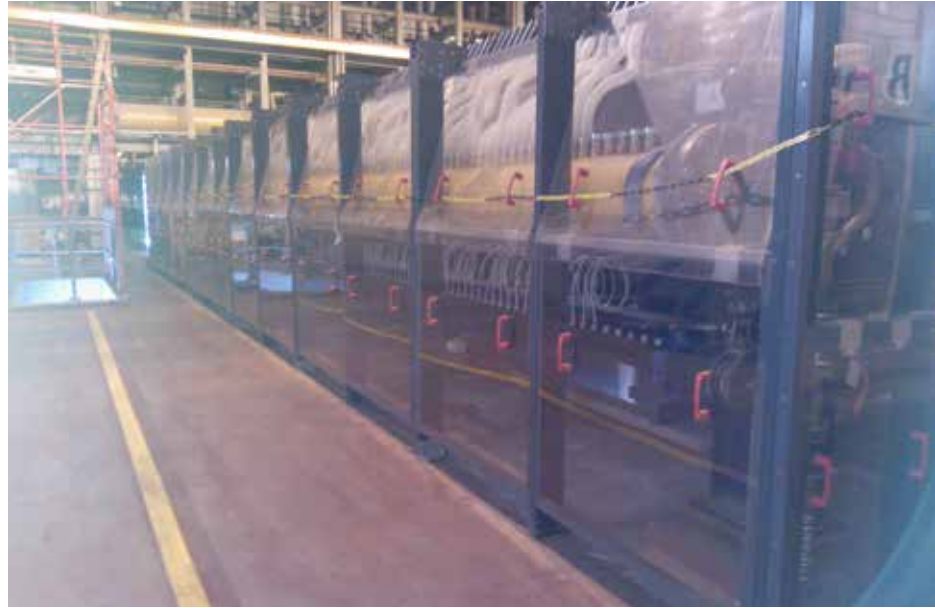
Figure 3.1 — Electrolysers in the cell room
