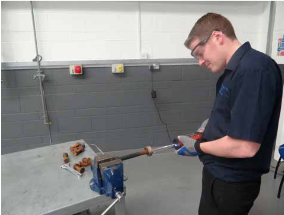
Figure 6.3 — A 1 kW hand-held induction heater being used to heat a seized bolt
