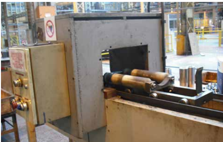
Figure 5.2 — Demagnetiser with sliding trolley
