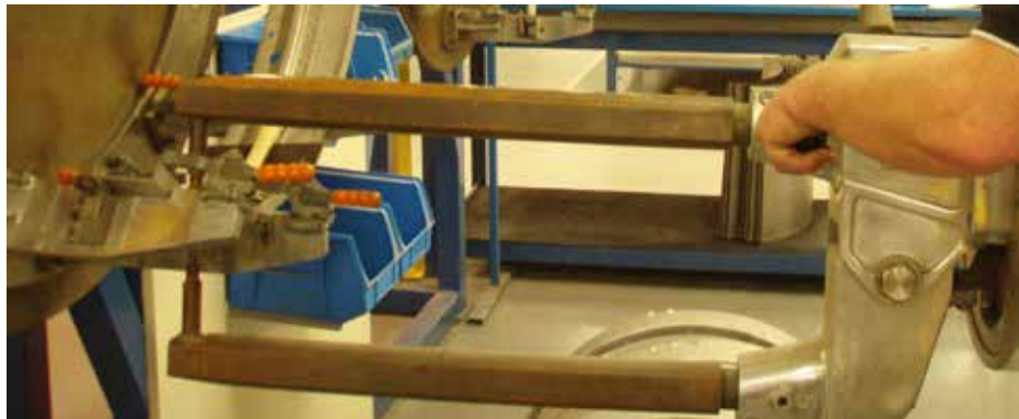
Figure 7.2 — Portable suspended spot welder
