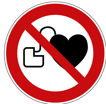
Figure 7.10 — Examples of warning notices for strong magnetic and an illustration of the prohibition symbol for AIMD wearers
