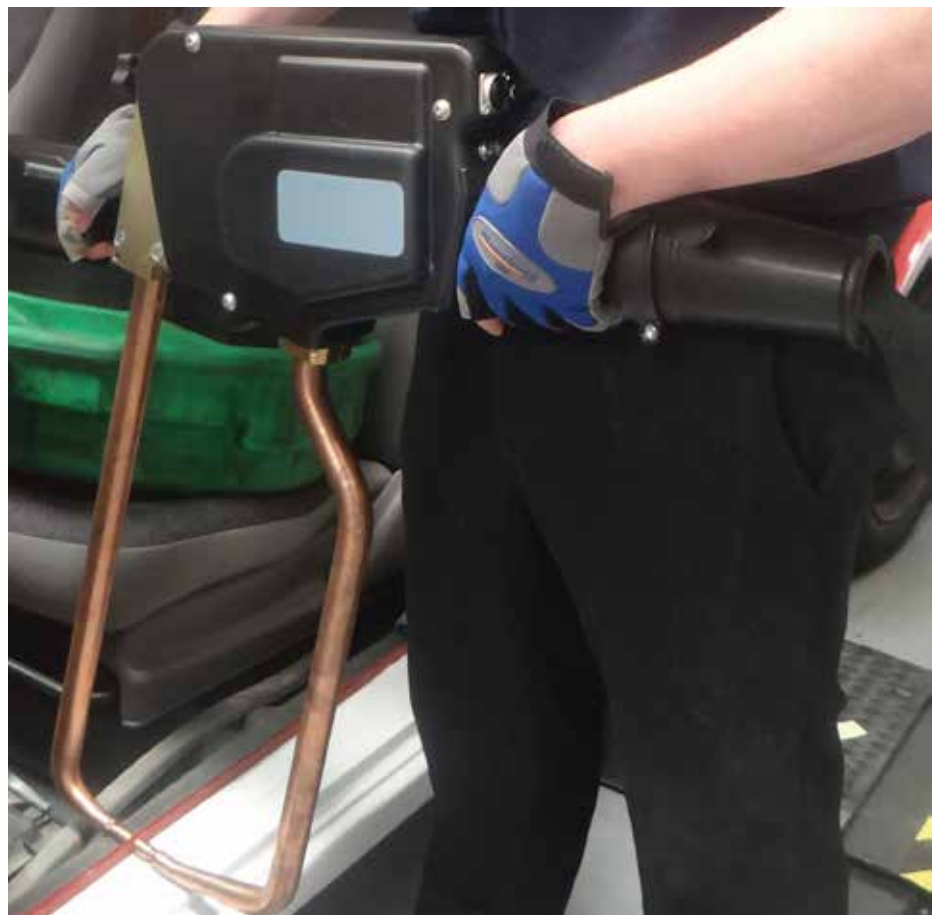
Figure 6.5 — The repair shop ‘X-type’ welding gun, with 550 mm electrodes fitted. The two electrodes are forced together in a pincer action by a piston in the main body of the gun (between the worker’s hands), which also contains the transformer supplying the welding current
