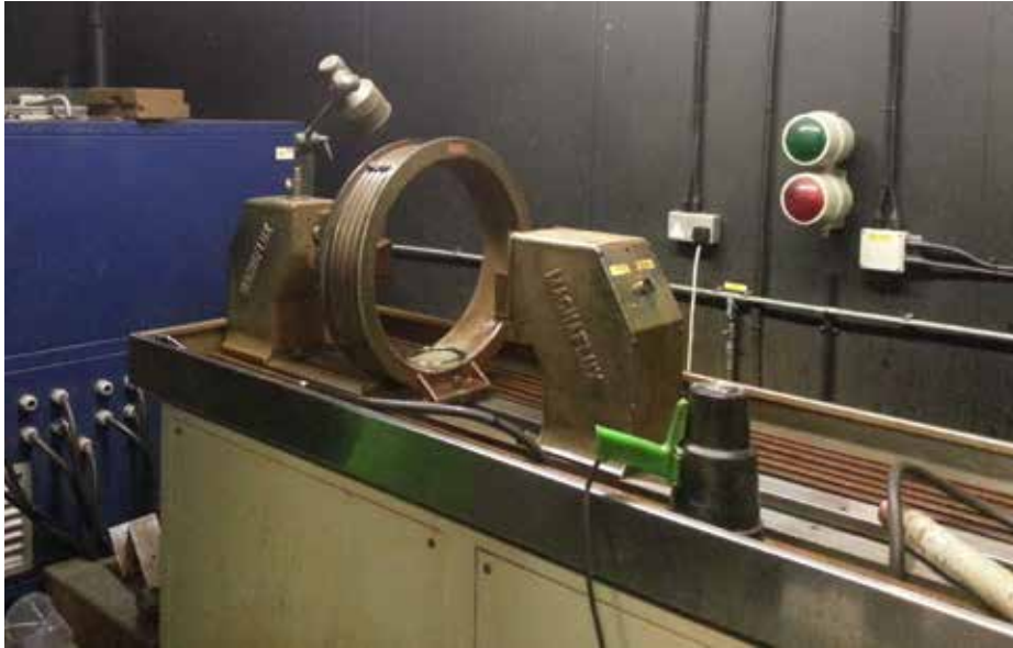
Figure 5.1 — Magnetic particle inspection unit
