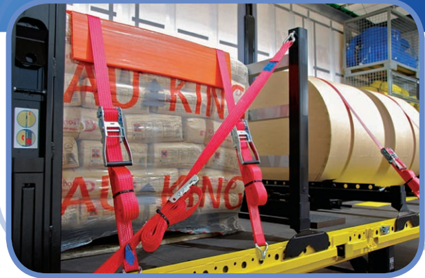
Figure 8. Example of an edge protector spreading the tie-down force on a unitised pallet load.
