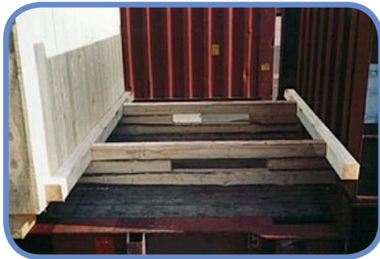
Figure 10. Example of a load blocked back from front with timber dunnage
