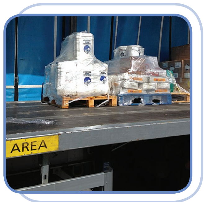
Figure 3. Unacceptable, unsecured pallets within a curtain-sided vehicle.
