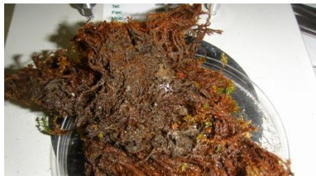
Figure 1: Discolored Chrysotile (white asbestos) probably as a result of thermal degradation
