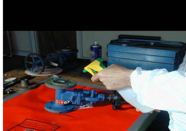
Dampening the asbestos gasket on a valve
