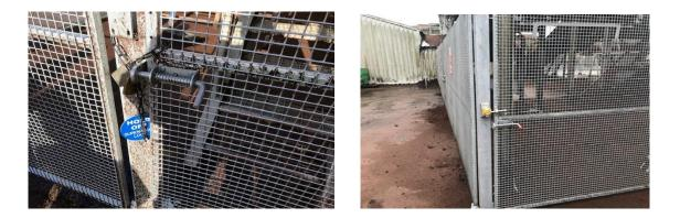
Modern captive key locking systems require the power to a piece of equipment to be isolated before allowing the key to be removed. The key should only be available if removing it from the electrical supply panel switches off the equipment and it cannot be energised without replacing the key. The key can then be used to open a gate or allow access to a paddle mixer/block maker or be retained by the person carrying out maintenance on the equipment.
