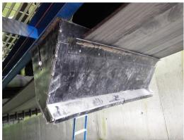
The feed hopper is the collecting device at the delivery point of the conveyor for receiving material.
