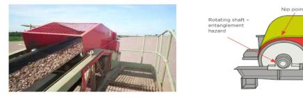
Tail/return drum guarding should enclose all rotating shafts and nip points and extend at least 600 millimetres from the entanglement hazards. They must require a tool to remove them and must be replaced following any maintenance work or clean up before the conveyor is restarted.
