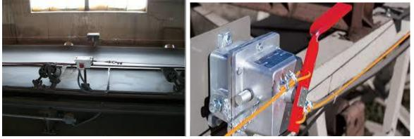
Emergency stop buttons are designed to stop the conveyor in the event of an emergency. Emergency stop buttons must be red, prominently marked and easily identified with a mushroom head latch in type or lock in type with manual reset; they should be tested on a regular basis.
