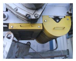
A scraper is a cleaning device fixed or flexibly mounted on the return (empty) side of the belt across the width of a belt or pulley of a conveyor, for removing material and require guarding if they are accessible and are a nip point.
