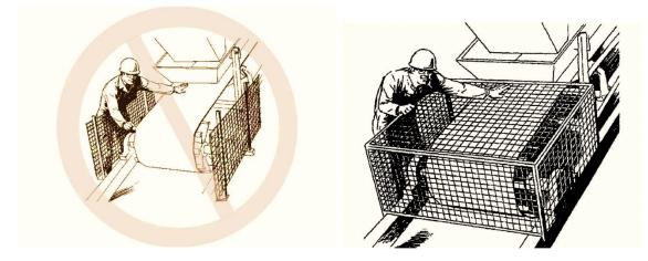
Drive belts transmit the power from the electric motor to the drive, they rotate at high speeds and should be fully enclosed and must require a tool to remove them and the guard should always be replaced following maintenance.
