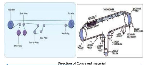
Head drum guarding should prevent access to head drums and all associated nip points. The distance from the guard end to the centre shaft of the head drum should be a minimum of 1000mm. Where troughing idlers are positioned close to the head drum and place the belt under tension, the guard should be extended.
