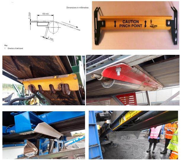
It is highly recommended that where any return idler roller is accessible and there is downward pressure on that roller that it should be enclosed or fitted with a guard that will prevent the trapping or crushing risk either in addition to or as a replacement for a nip guard. Examples of suitable idler roller guarding are shown below
