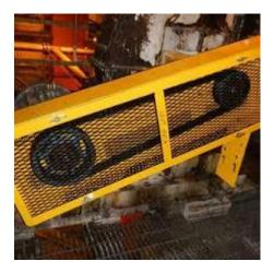
Vertical tension Units must be guarded at the top and the bottom of the tensioner. At the top the guard must extend at least 600 millimetres beyond the nip point.
