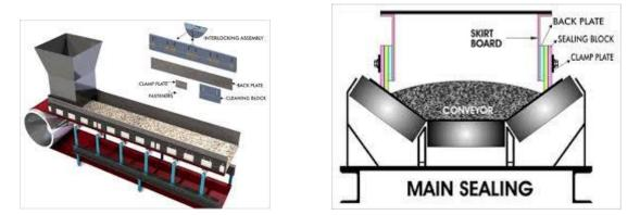
A chute is a straight or curved, open topped or enclosed, smooth trough through which materials are directed and fall under gravity onto another conveyor, crusher, sizer, screener or stockpile.
