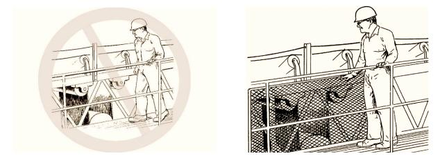
The area at the base of the tension unit must prevent access to any nip points or rollers and be of adequate height to prevent anyone reaching into the unit as shown on the illustration on the left below.
