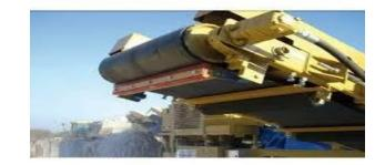
Return idler rollers support the return (empty) side of the belt and require guarding if they are accessible and have downward pressure placed upon them by the conveyor.
