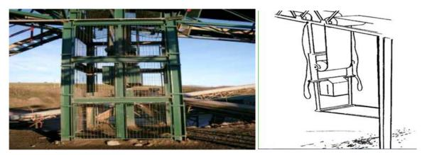
Conveyor vertical take up device takes up slack and applies tension to the conveyor belt, particularly at start up or during heavy loading. Normally a vertical weight moves up and down to apply the tension.
