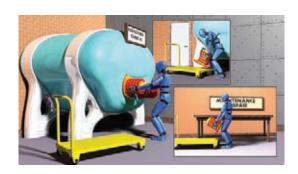
and lifts it from the machine onto the trolley. He then transfers the part on the trolley to the workshop. The part is then lifted off the trolley to a workbench for the maintenance work to be completed.
